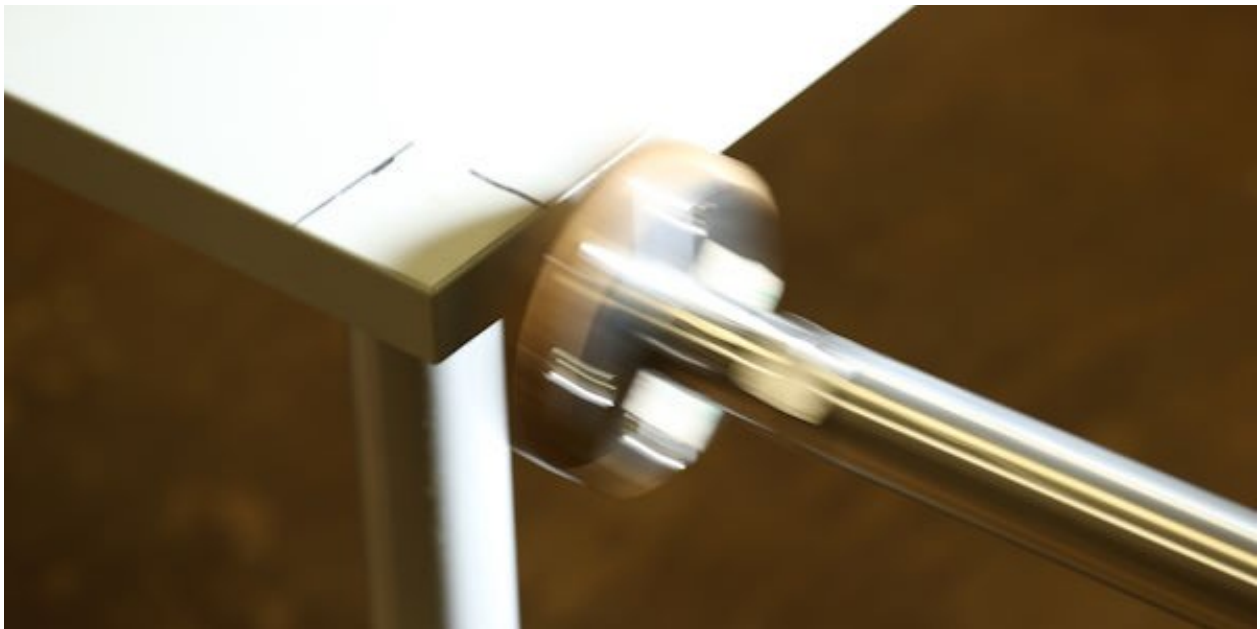
A horizontal durability test is undertaken to show the strength and durability of the table
