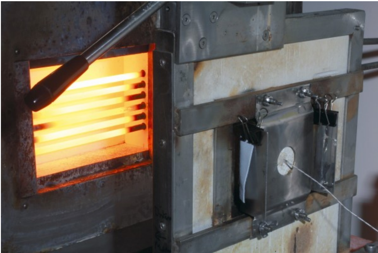
Figure 3: The radiant heat test
